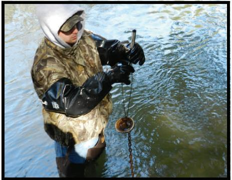
*To protect the datalogger from damage, it is attached to a chain in the pipe.*
